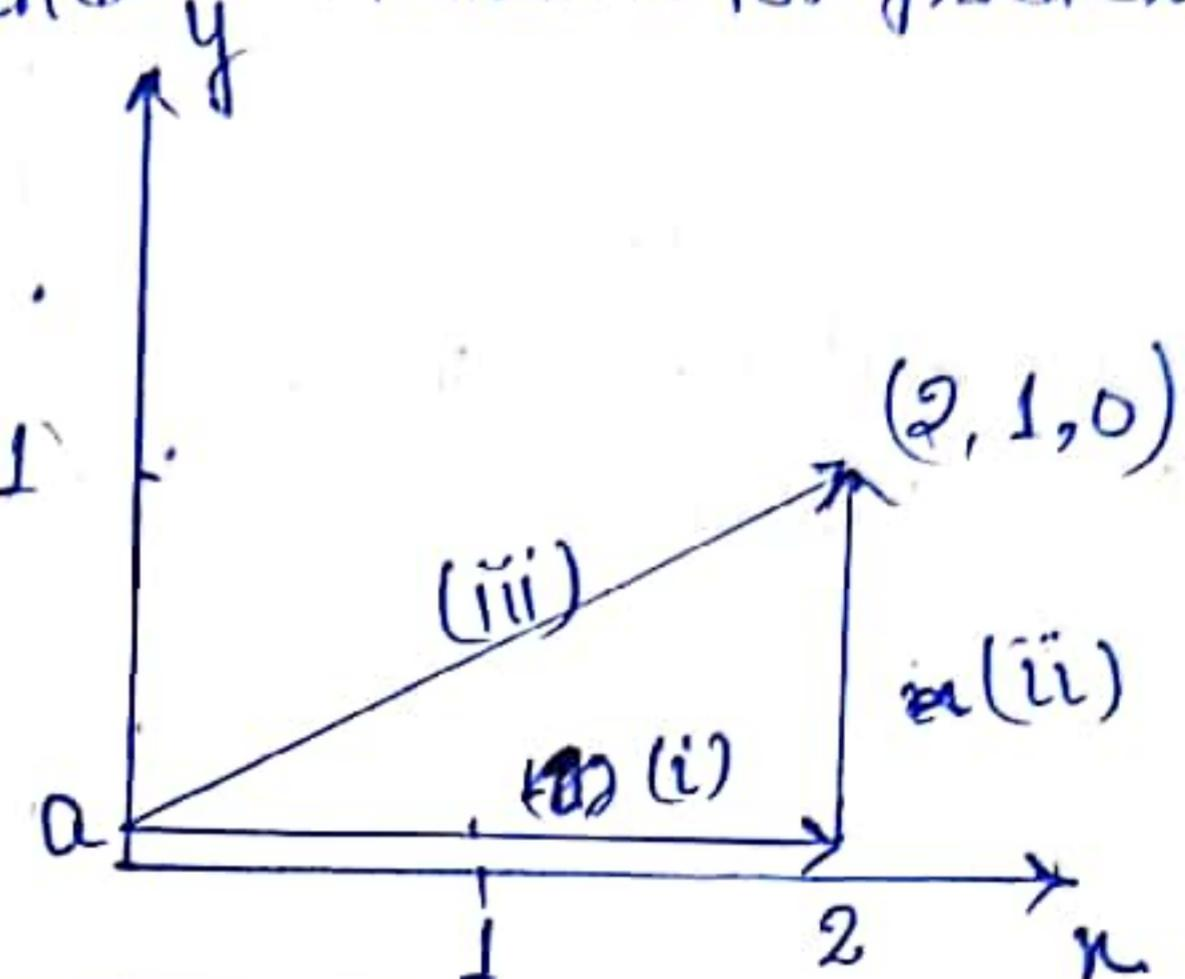
$$\begin{aligned} &\int_0^1 y^2 dy \hat{x} \cdot \hat{y} + \int_0^1 4y dy \hat{y} \cdot \hat{y} \\ &= \int_0^1 4y dy = 4 \left[ \frac{y^2}{2} \right]_0^1 \\ &= 2 \end{aligned}$$
