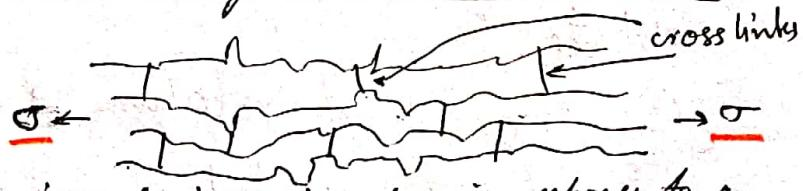
② during elastic deformation in response to an applied tensile stress.
