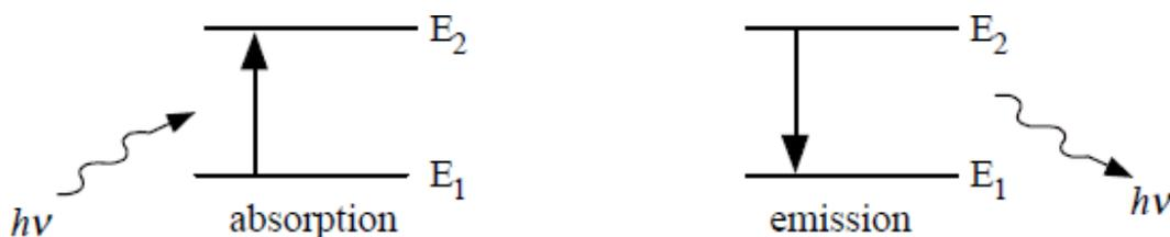
Flame photometry or flame emission spectroscopy is an atomic emission technique. There is no need for light source. Flame serves both as an atomizer and excitation source. It is suitable for qualitative and quantitative determination of several cations, especially for metals that are easily excited to higher energy levels at flame temperature. These metals are Na, K, Ca,
