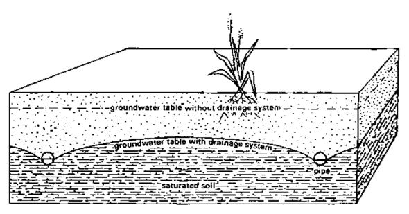
Figure 4. Pipe drains
