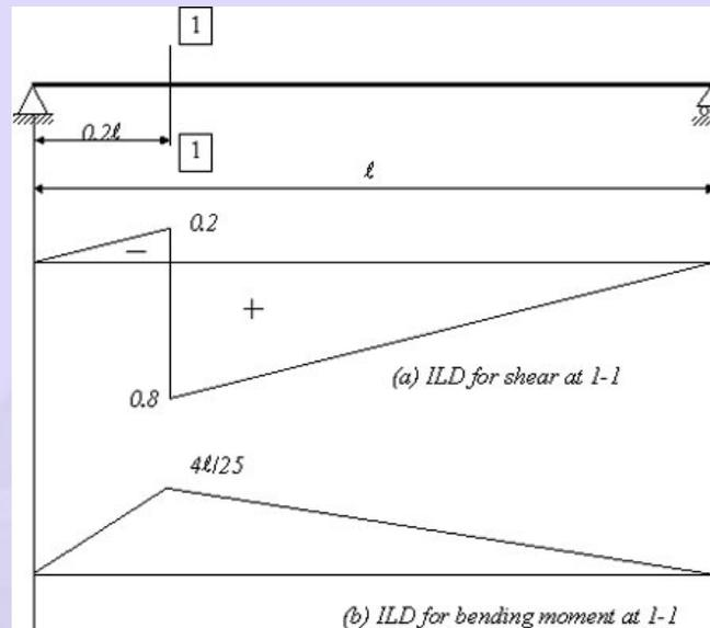
**Fig. 7.12 Influence lines for shear and bending moment**
